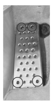
Place the self-tapping screws into the locations shown and use the Phillips screw driver or power drill with Phillips attachment to properly mount the footrest.
