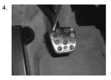
Using the bolt and locking nut, secure the brake & clutch pedals using a Phillips screw driver and 7mm socket wrench to tighten.
