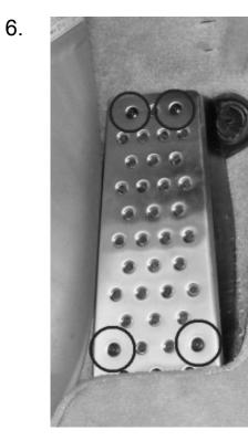
Place the self-tapping screws into the locations shown and use the Phillips screw driver or power drill with Phillips attachment to properly mount the footrest.
