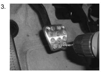
Place one of the brake/clutch pedals over the clutch to use as a template. Using the provided drill bit, drill the 3 holes needed.
