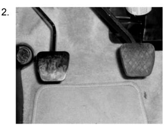
Remove the stock rubber pads on the brake & clutch pedal.
