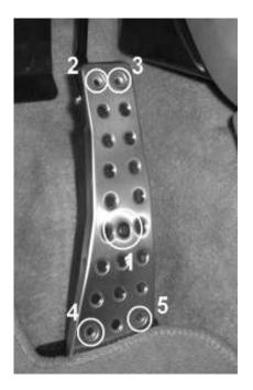
Place the stainless steel gas pedal cover over the existing plastic pedal. Using the Phillips screw driver or power drill, install the first self-tapping screw into the middle location 1. Once location 1 is installed, proceed with locations 2 through 5.
