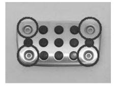
Remove the stock rubber pads on the brake pedal and place the brake pedal with rubber insert onto the pedal. Drill the 4 holes into the brake pedal and install with the bolts & locking nuts
