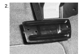
Remove the stock rubber pads on the brake pedal.
