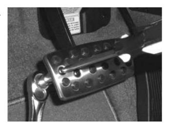
Using the bolt and locking nut, secure the brake pedal using a Phillips screw driver to hold it in place and 7mm socket wrench to tighten.
