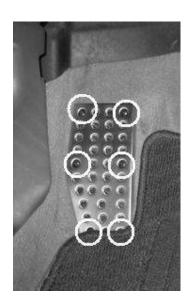
Place the stainless steel footrest over your existing footrest and use the self-tapping screws to install on the locations shown on the picture. Use a Phillips screwdriver or a power drill with Phillips attachment to properly mount the footrest.
