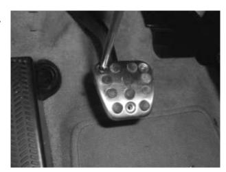
Using the bolt and locking nut, secure the brake & clutch pedals using a Phillips screw driver and 7mm socket wrench to tighten.
