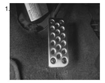
Place the stainless steel gas pedal cover over the existing plastic pedal. Using the power drill, drill 4 holes where at the mounting locations on the pedal. Install the two self-tapping screw onto the top locations. The bottom two holes require the use of the longer bolts & nuts. They should extend out the opposite end just enough for the nuts. The self tapping screws can be used on the bottom two mounting locations but the use of nuts & bolts are highly suggested.
