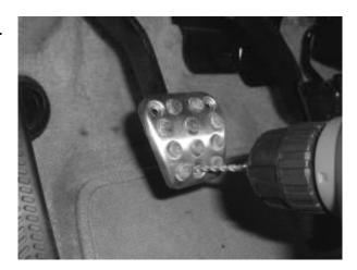
Place one of the brake/clutch pedals over the clutch to use as a template. Using the provided drill bit, drill the 3 holes needed.
